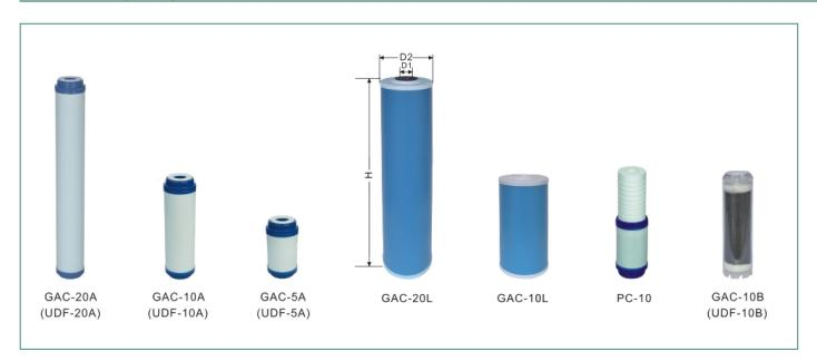
The granular carbon filter cartridge is made of the granular carbon media, such as: coal carbon, fruit shell carbon and coconut carbon, and the food grade housing. It can remove the chlorine, taste and odor from the water. According to the requirement, various types and sizes are available for option.
