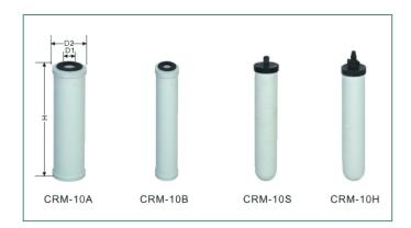
The various ceramic filter cartridge is sintered by the special material. This cartridge has less than 0,2 micro filtration precision, can remove harmful substances such as: dust, particles and bacteria. It has high flowrate, long service life and chemistry stability. The advantage of this cartridge is that it can be washed with brush when cartridge is dirty.
